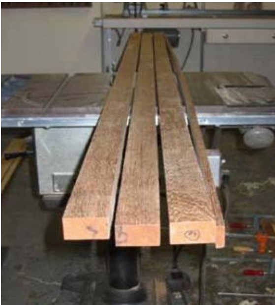
Figure 1 - Teak Board after first ripping
