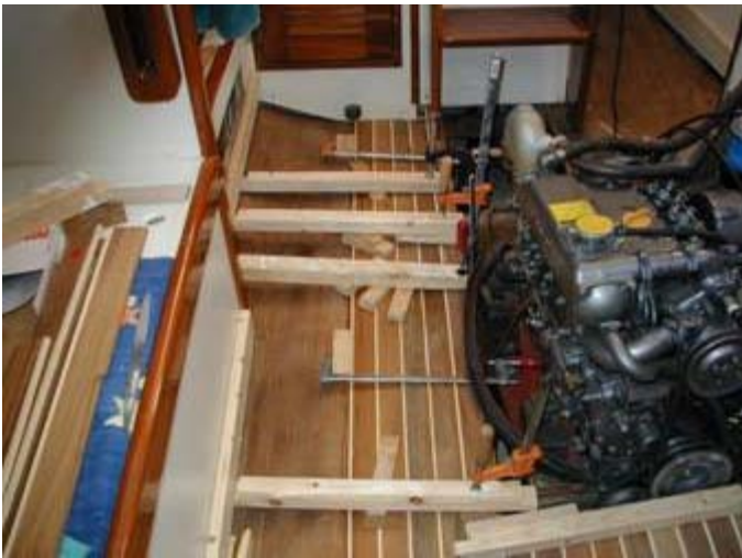
Figure 12 - Clamping planks in galley area
