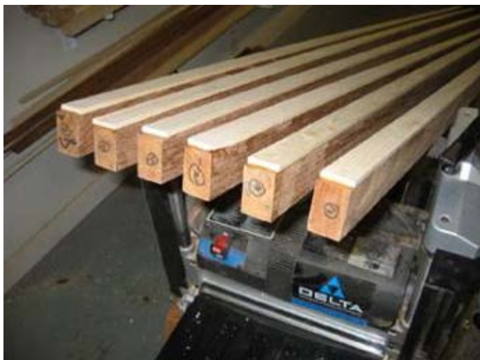
Figure 2 - Aspen strips glued on teak ready for 2nd ripping
