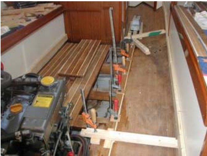
Figure 11 – Aligning plank with bilge edge to start starboard side
