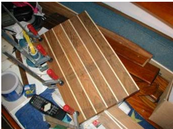
Figure 6 - A bilge board being clamped
