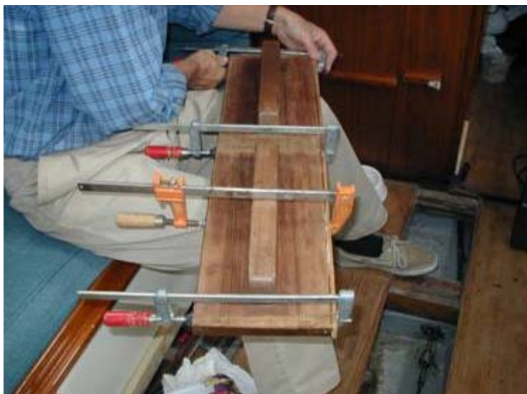
Figure 4 – Shims are placed on bilge board and clamped
