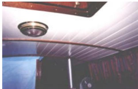
Next, however, comes the part you've been waiting for. Put your first plank along the centerline of the roof. Screw it to the plywood battens. Be sure to line the screws up so they will be hidden by the athwartships splines you will be putting back. Keep doing this until you reach the edges. The last planks will have to be shaped to fit along the curvature of the roof. It doesn't have to be perfect as you're going to cover
