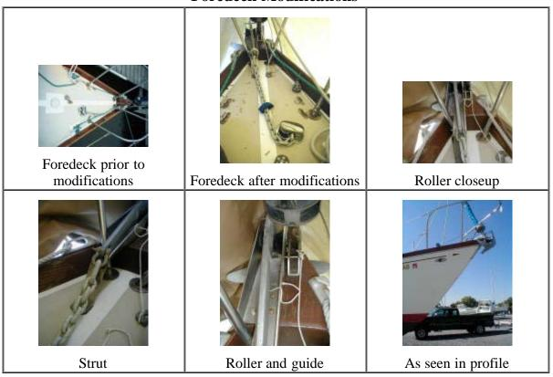
• Recommended technique for a split chain anchoring system.
